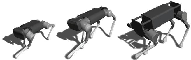
Fig. 4: Using our control pipeline, animal-like motions can be reproduced by various robot models with different scales and actuation power. We ran experiments with three robotic platforms from *Unitree: AI* [14] (**left**), *Aliengo* [12] (**middle**) and *Laikago* [15] (**right**).
